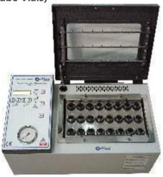
Nitrogen Evaporator Model: **AT-EV-24** is a Precision Sample Concentrator by Nitrogen Purging. It is a newly designed Sample Concentrator for multiple sample pre-concentration of in organic media for Vortex Motion Concentration and ASE (Dionex) Compatible upgrade Kit (For I-Chem vial 40mL, 60mL). A Table Top Model. The unit can be set to a constant Flow and constant Temperature to ensure good evaporation.
